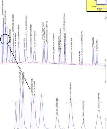
The DELCD chromatogram is shown at left in more detail, and with the peaks labeled for identification. The DELCD is completely selective for compounds containing chlorine and/or bromine. Other analytes do not respond at all, even at very high levels. The DELCD actually operates on the FID's exhaust gases; therefore, all contaminants are pre-combusted by the FID to CO<sub>2</sub> and H<sub>2</sub>O.
