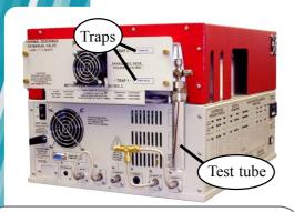
The Method 5030 Compliant Purge & Trap uses disposable test tubes at ambient temperature.
